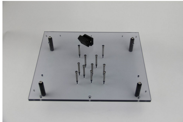
Cassette top-plate (push-finger plate): the transparent plate with pushers.
